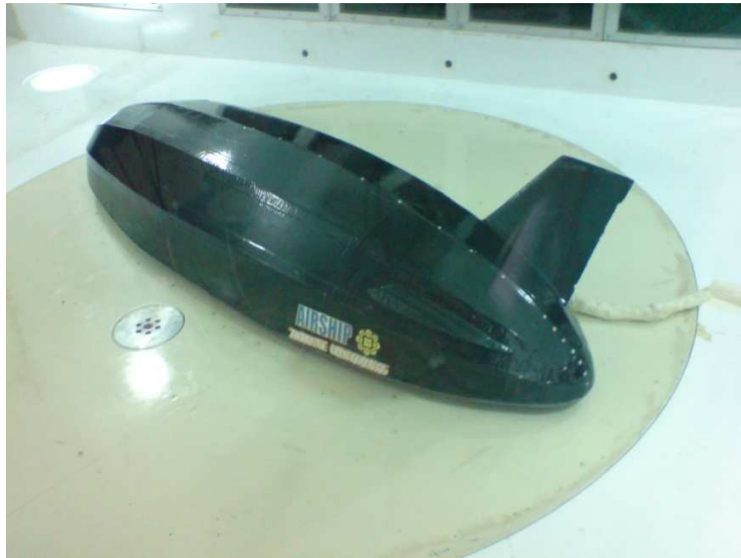
Figure 36-6 Pressure measurement testing at 25° angle of attack
