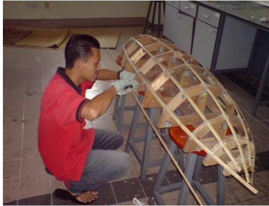
Figure 34-9 Attaching bamboo stick to the frame structure
