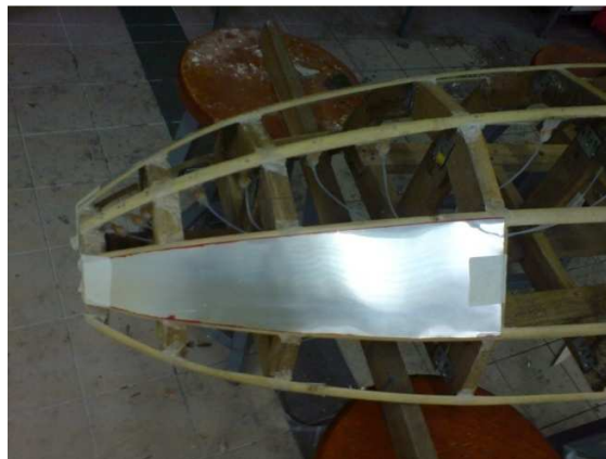
Figure 35-3 Tail support attachment
