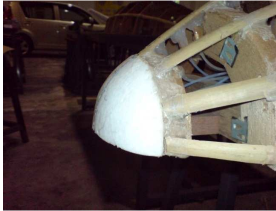
Figure 35-6 Front bow cap attachment
