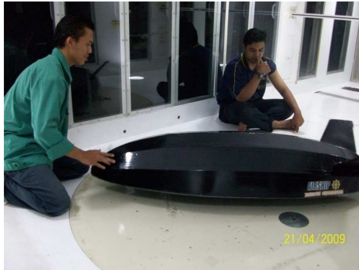
Figure 36-3 Installing the model in the test section
