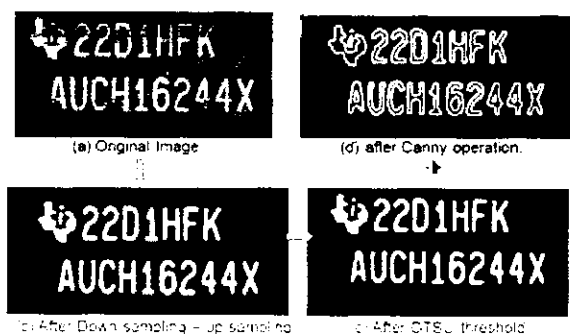
Fig. 1. A sample IC marking image after each preprocessing operation
