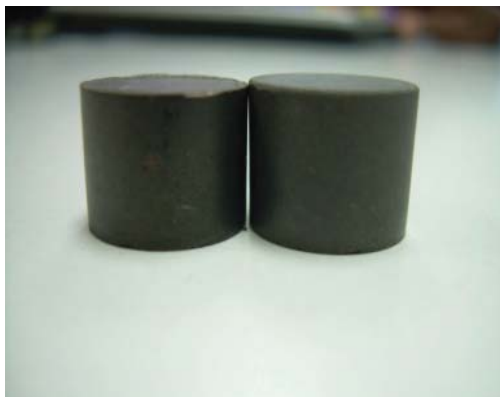
Fig. 3 Electrodes sintered at 450 °C for 30 min.
