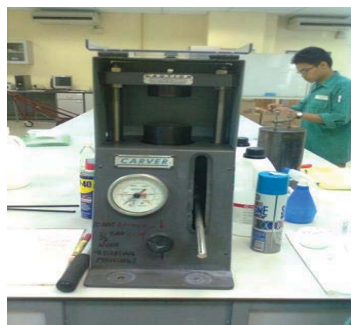
Fig. 1 The carver press used for compaction.
