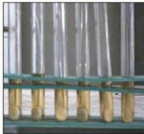
Figure 1. The disk specimens in BHI broth for the bacterial adhesion test.
