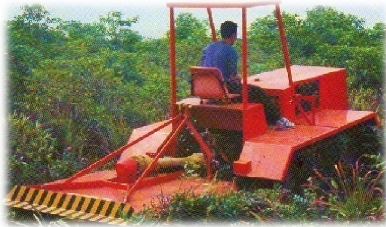
Figure 10.1. Peat tractor prototype (Source: MARDI, 1996 Report No. 184)
