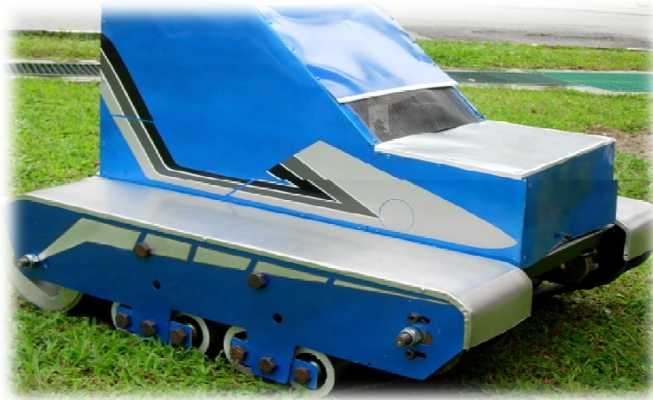
Figure 8.16: Developed air-cushion tracked vehicle.
