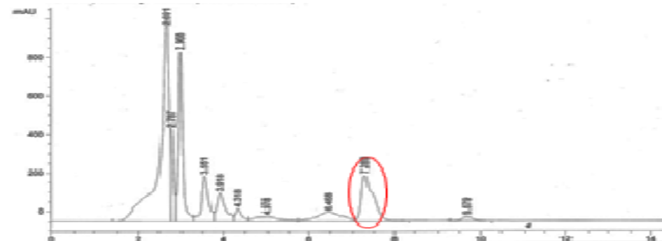
Figure 2. HPLC graph and peaks of retention times
