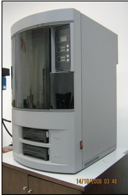
Fig. 8: Dimension SST 768 machine and its build material and support material
