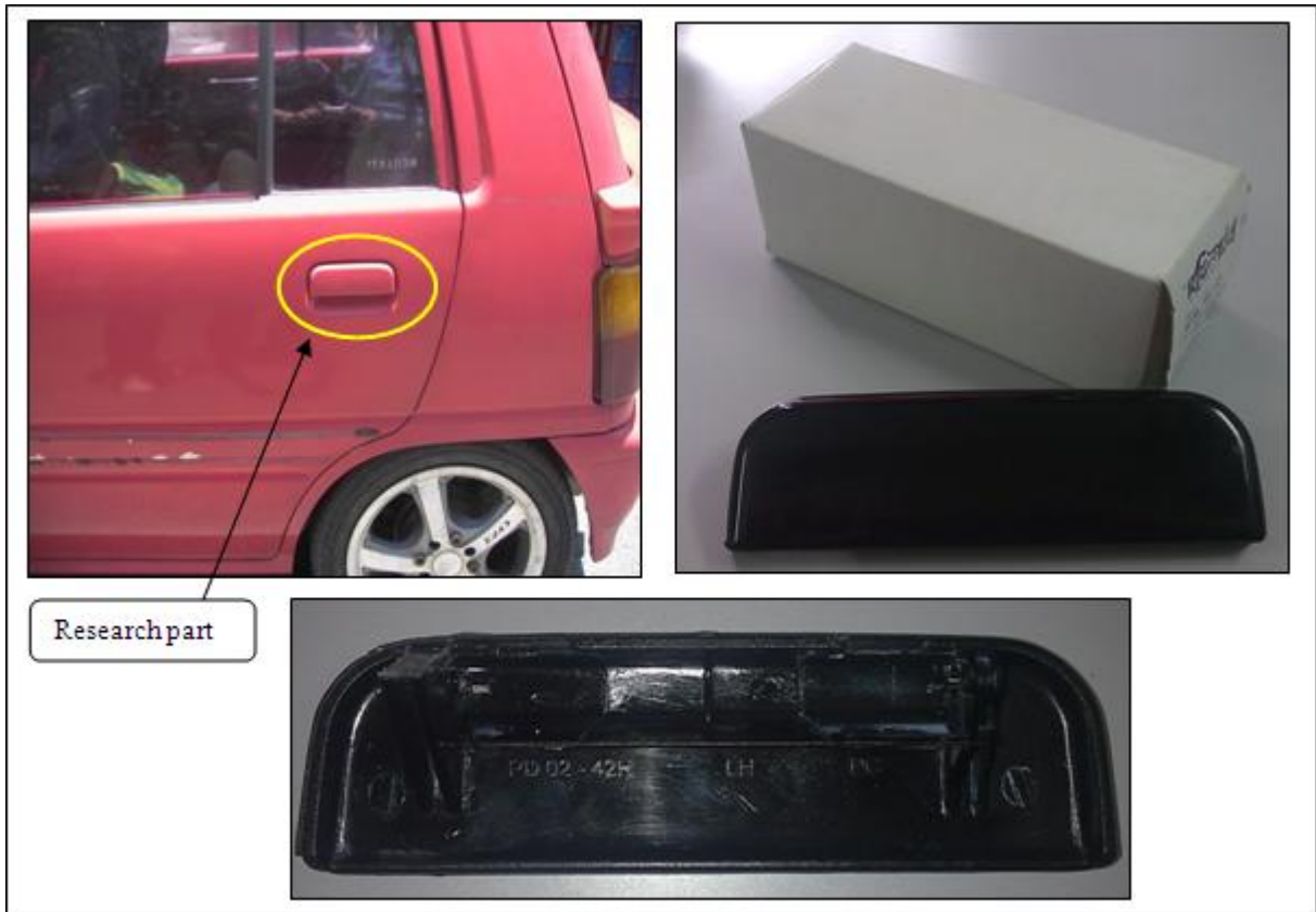
Fig. 3: Original Model of outer handle back left door of Perodua Kancil car model
