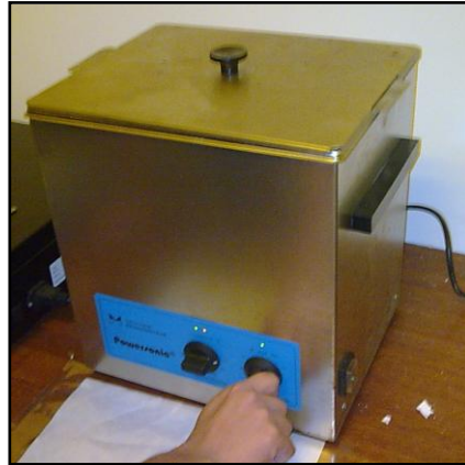
Fig. 17: Finishing part by sink the parts into container (about 70°C)
