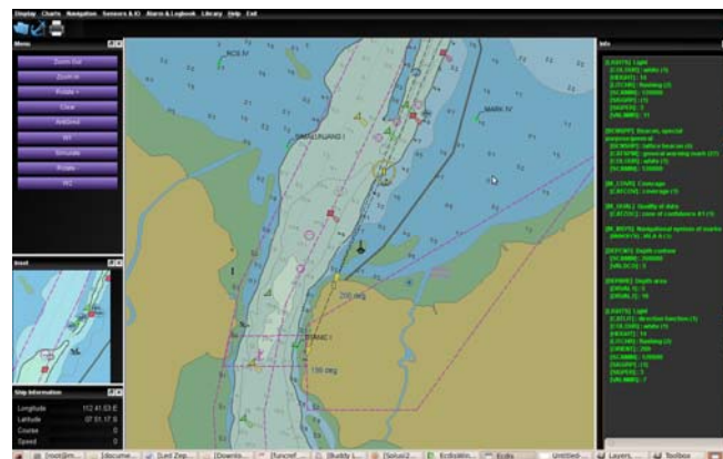
Figure 1. The main view of ECDIS application. It consists of three main windows. The main window, which displays the electronic chart, appears in the middle of the screen. The left window contains command buttons, chart inset, and information about the actual position of own ship. All related information about navigational objects or critical events during the seafaring are shown on the right window.
