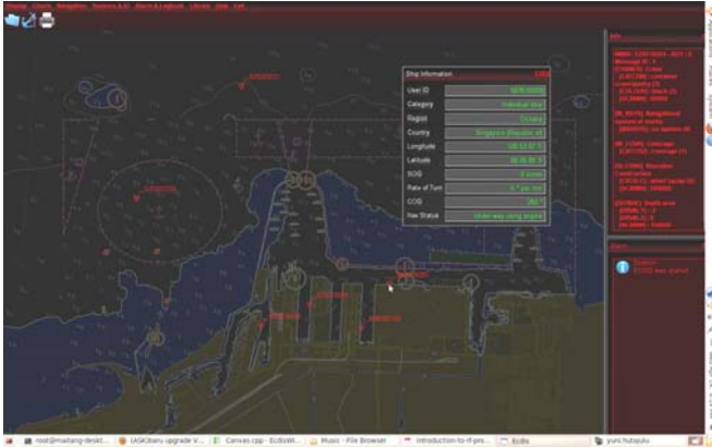
Figure 5. Display of ECDIS in the night color mode. Various color modes are available depending on the environmental situation on the vessel.
