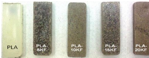
Figure 4 Photomicrographs of the PLA-KF biocomposite after burial for 40 days.
