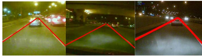
Fig. 12: Curved and straight road lane detection in a highway during night.
