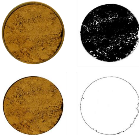
Fig.1: Estimation of soil shrinkage via digital image analyses (Software Image J Version 1.4).
