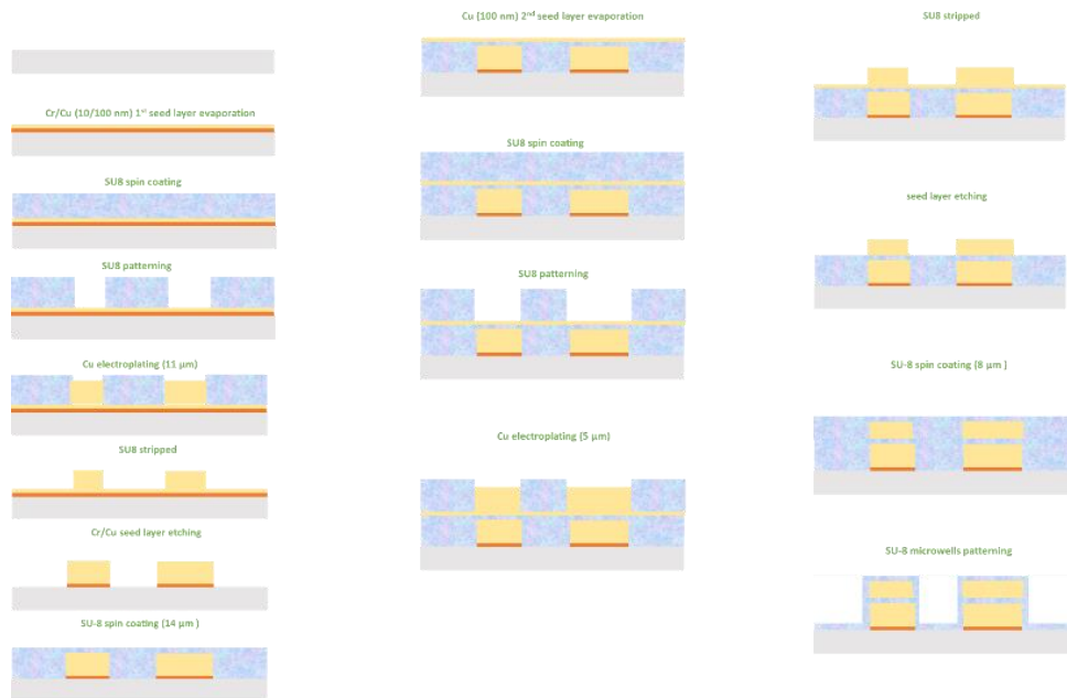
Figure 4.20 : Vertical electrodes fabrication process flow
