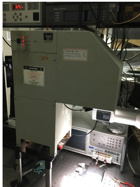
Figure 2.3 300 W Xenon lamp solar simulator.
