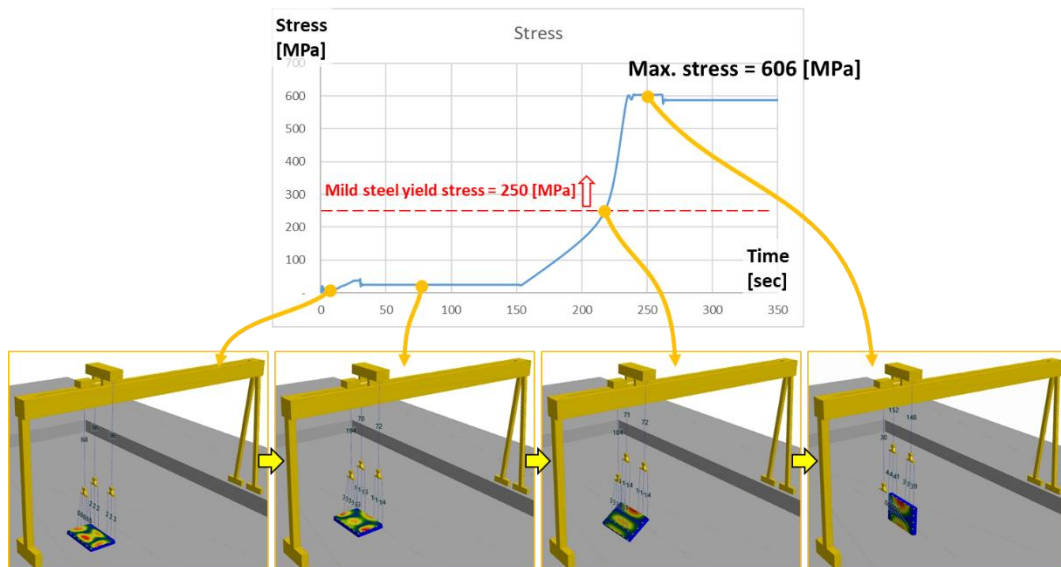
Figure 4-17. Graph of the maximum von-Mises stress.
