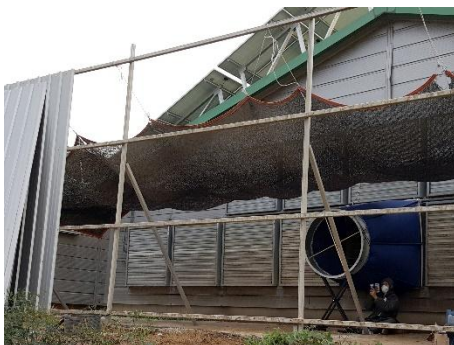
(a) Airflow measurement without windbreak
