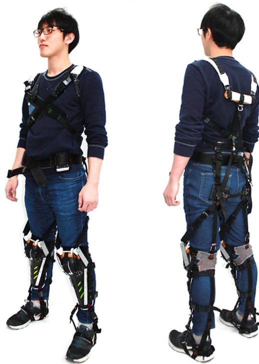
Fig. 2.1. Prototype of soft wearable device for lift assist
