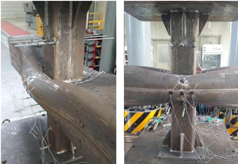
Figure 3.9 Chord plastification (X90-325-0.625-26.7)
