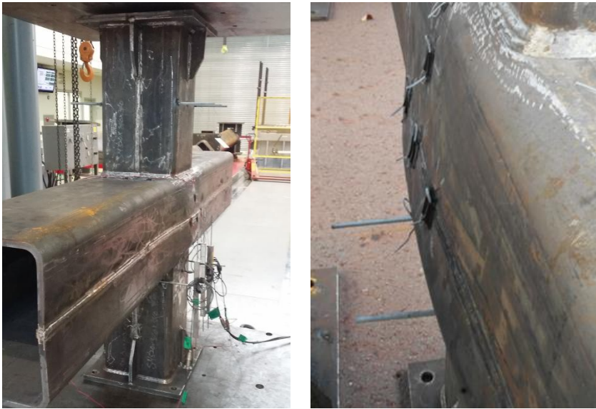
Figure 3.12 Bulging occurred at the mid-height of the chord sidewall (X90–325–0.850–26.7)
