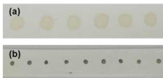
Figure 1-3. The photographs of AgNP spots on filter papers. (a) AgNP spots on bare filter paper and (b) AgNP spots on AKD-treated filter paper.
