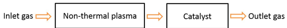
Figure 1-1. Schematic overview of two plasma-catalyst hybrid system configurations; (a) in-plasma catalysis (IPC) and (b) post-plasma catalysis (PPC).
