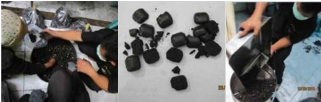
Fig 4-14 Photos of Briquette Drop Shatter Test (Sampling, Result of Drop, Measuring)
