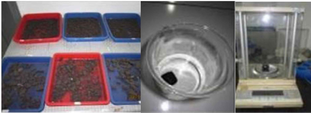
Fig 4-16 Soaking Test on the CUPO Briquette
