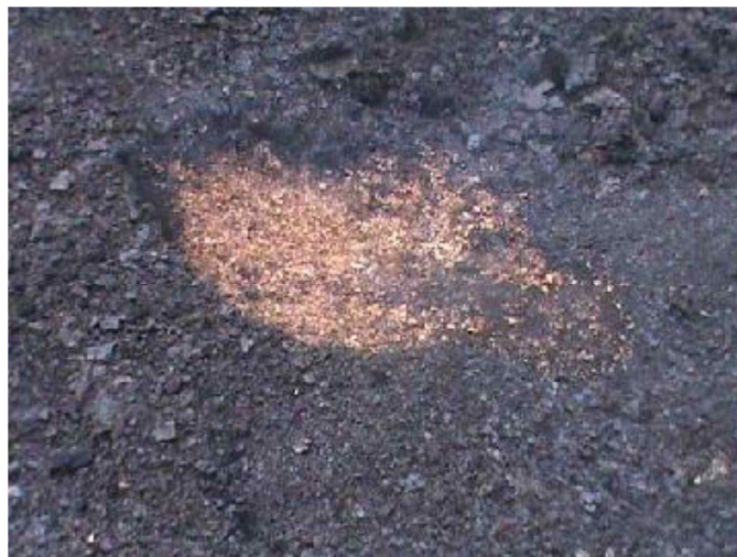
Fig 2-11 Spontaneous Combustion after 76 days of Stocking
