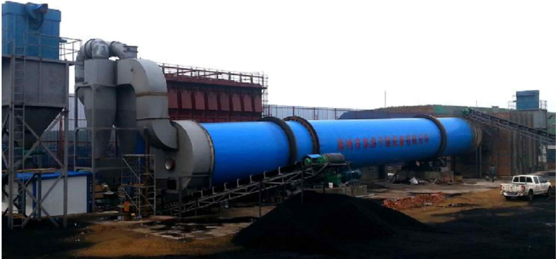
Fig 3-3 Photo of Direct Drying using Kiln Type Dryer #2
