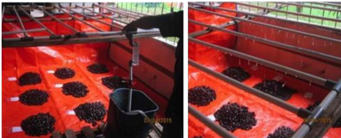
Fig 4-18 Extreme Rainfall Simulation of the CUPO Briquette
