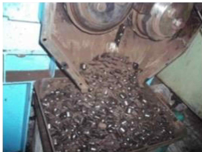
Fig 4-11 Photos of Taiyo K-102 briquetting machine and its briquette
