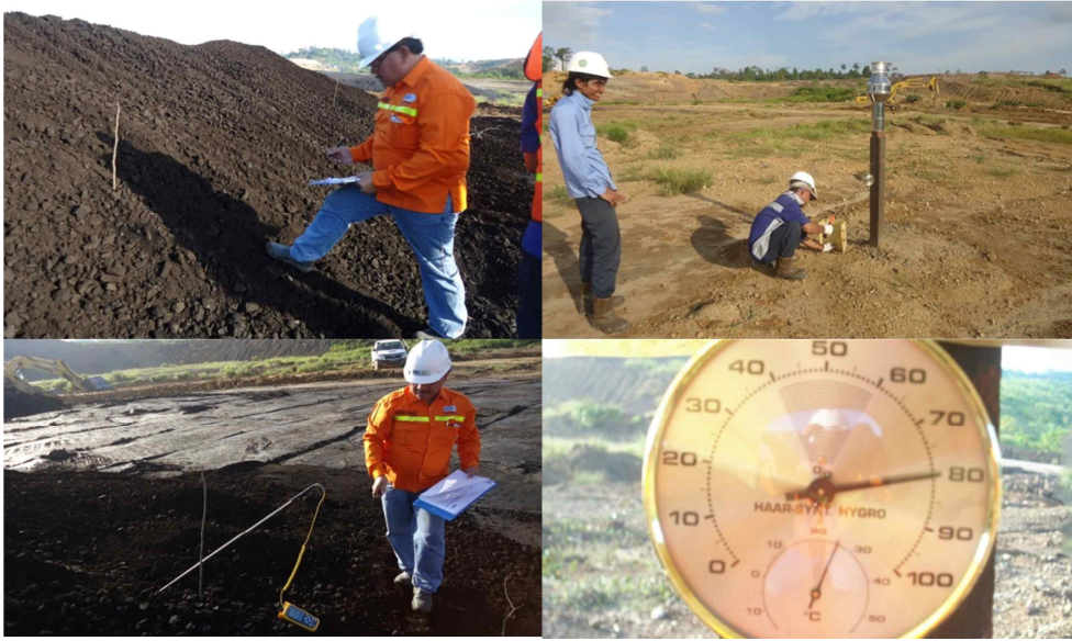
Fig 2-3 Opened Stockpile test - Temperature Rain & Humidity
