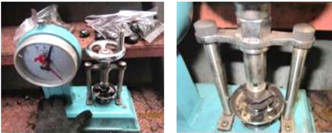
Fig 4-12 Photos of Briquette Strength Test
