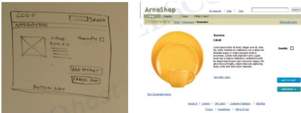
Figure 12. Low-fidelity prototyping (on the left) and high-fidelity prototyping (on the right) (Arnowitz et al., 2010)
