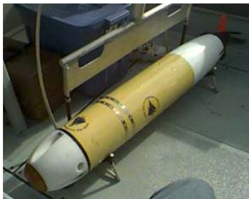
Figure 9. The REMUS 100 Autonomous Underwater Vehicle (T.Presto, 2001)
