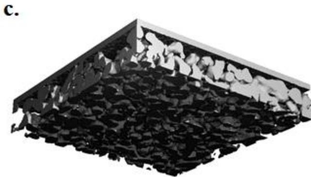
Fig. 2 Previous research which show that ice asperities are flattened by sliding. (a) Ice surface was observed with LT-SEM after being rubbed with steel(Ref. 24), (b) Flat Perspex surface coated by soot is rubbed with an ice rod and observed by microscope.(Ref. 4), (c) a layer of compacted snow is observed by MicroCT.(Ref. 8)
