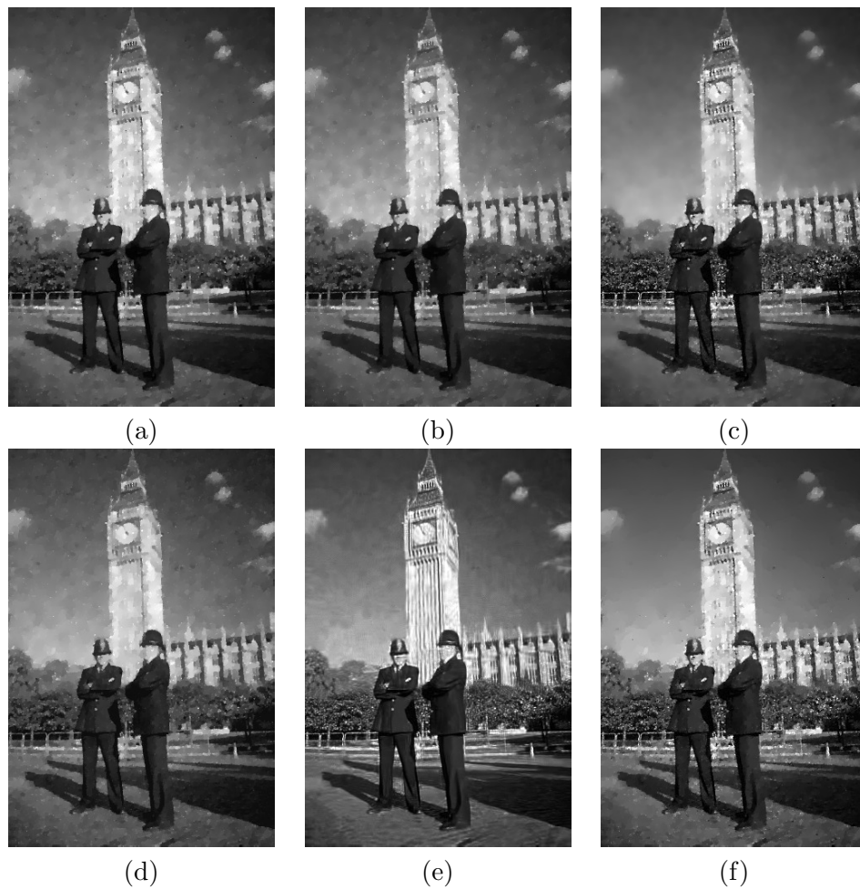
Figure 3.5: Denoising results of our model when M = 5 and comparisons with the exp [48], SO [65], TV-SARP [17], TwL-4V [35], SAR-BM3D [59] models. Denoised images with PSNR values: (a) exp (23.82) (b) SO (23.63) (c) TV-SARP (24.01) (d) TwL-4V (23.78) (e) SAR-BM3D (25.14) (f) our model (24.21)
