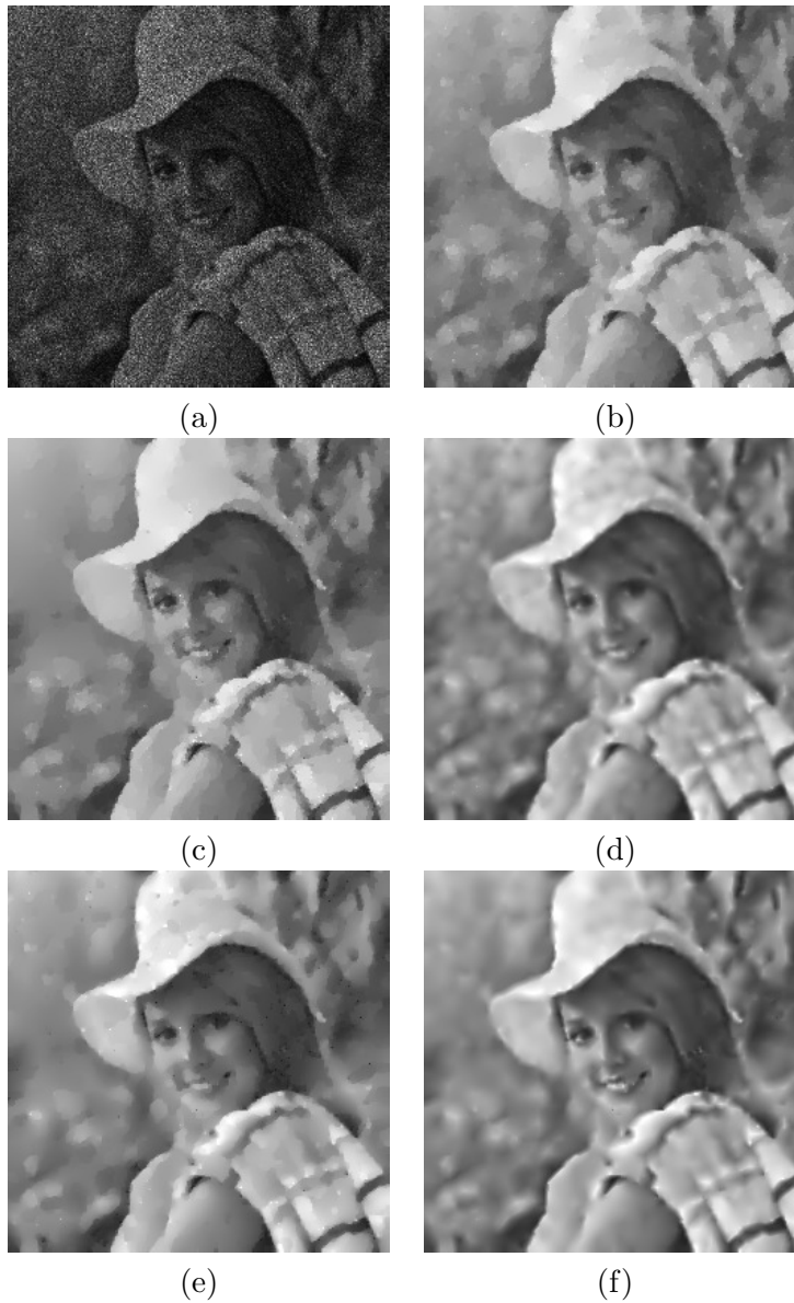
Figure 3.19: Denoising results of our model when M = 10 , and comparisons with other models: (a) data f with M = 10 . Denoised images: (b) TwL-4V [35]; (c) exp-SARP [51]; (d) SO-TGV [25]; (e) DZ-TGV [64]; (f) our model.
