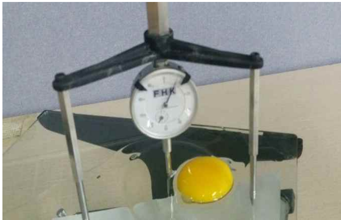
Fig. 5-1 Measurement device of the Haugh unit.
