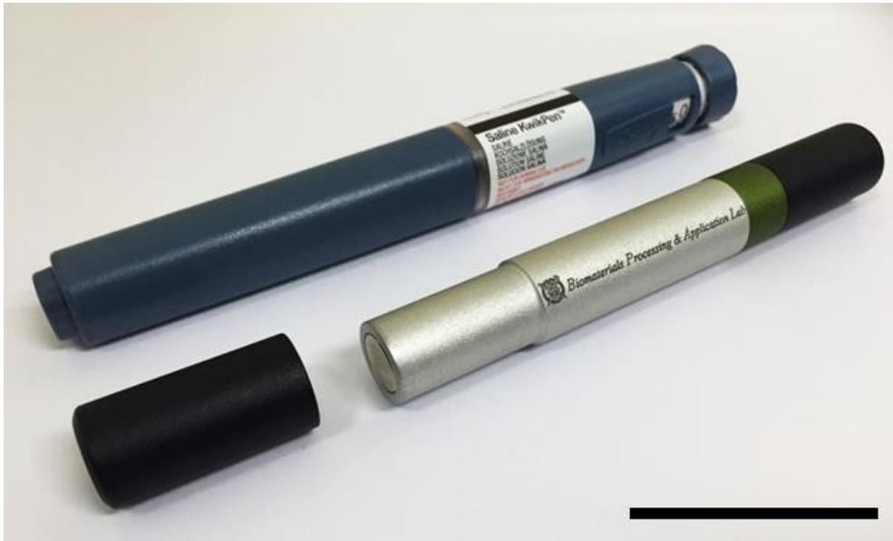
Figure 3.6 Image of a commercial insulin pen and the external device prepared in this work. I designed an external device closely following the size and shape of an insulin pen approved for clinical use (KwikPen®, Eli Lilly, USA). The scale bar is 5 cm.
