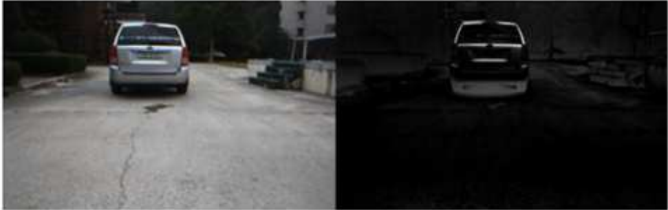
Figure 2.5: Original image and the result image through the high-pass Gaussian filter. The pixel value gets brighter around the boundary of the object.
