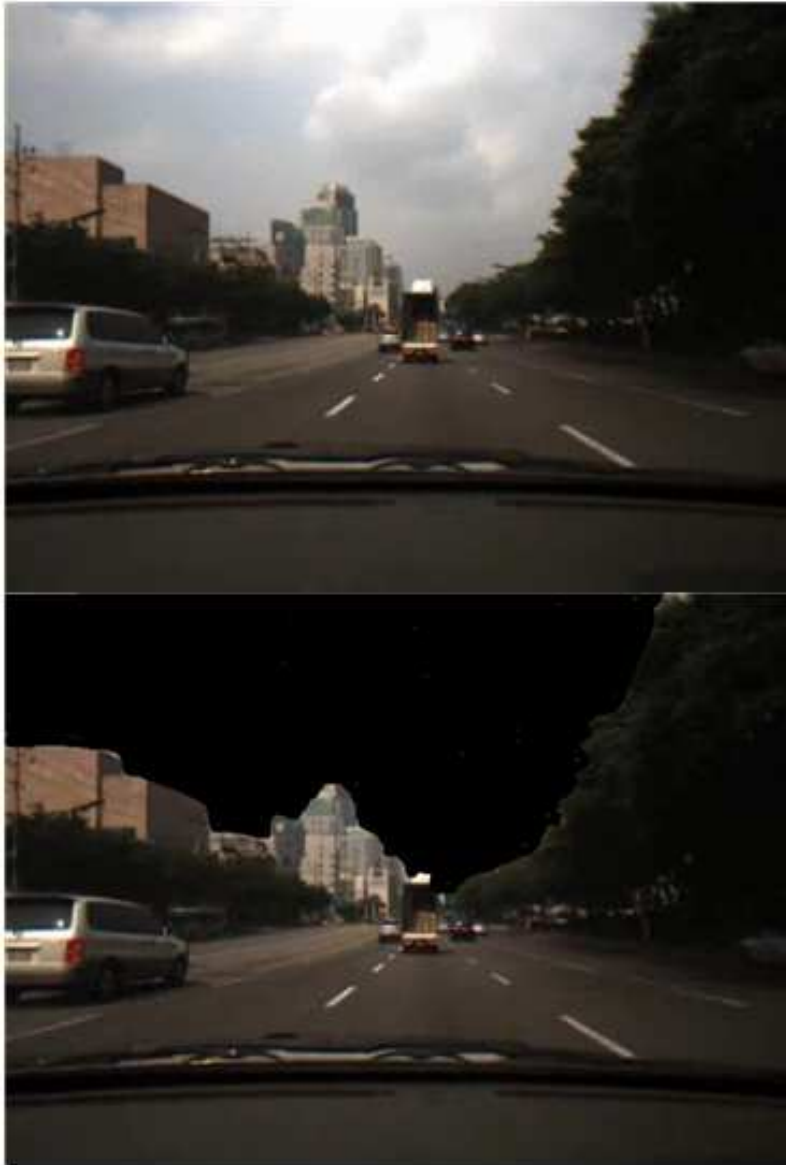
Figure 2.4: Comparison of an original and the same image with the sky removed (shown in black). Based on the image with the sky removed, the region of interest is reduce when generating the disparity map.
