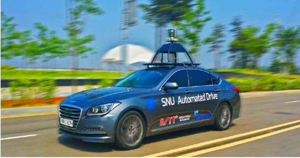
Figure 3.7: Autonomous vehicle equipped with a 3D LIDAR for generating map. monocular camera is mounted on the location of rear-view mirror in the vehicle.
