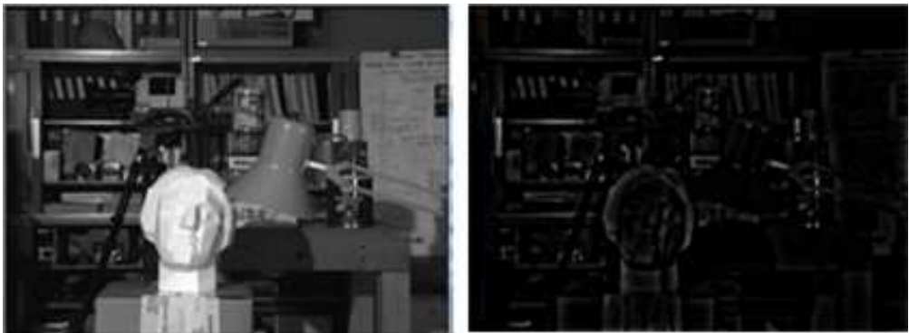
Figure 2.6: Original image and the result image through the high-pass Gaussian filter. The pixel value gets brighter around the boundary of the object.
