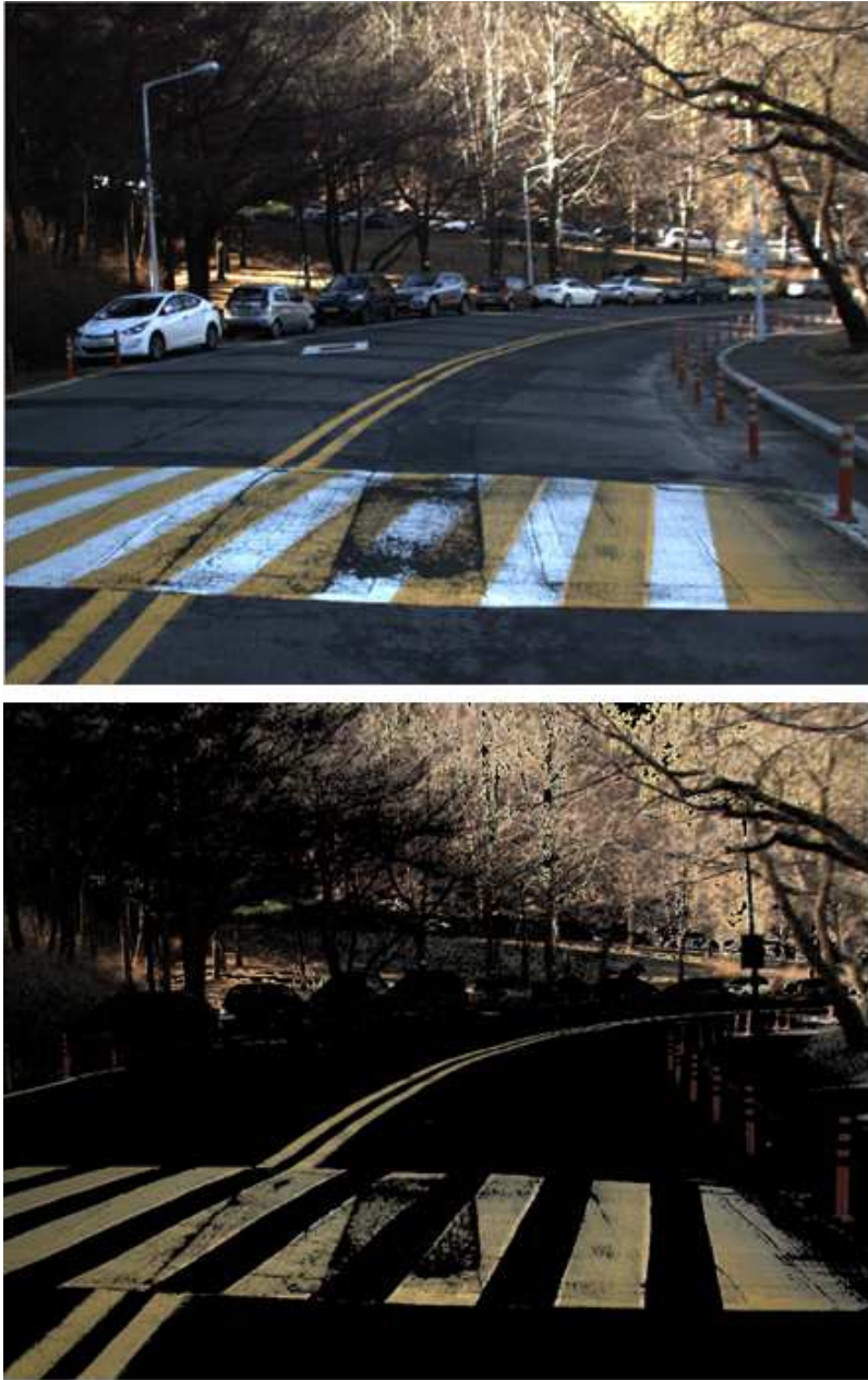
Figure 3.5: Example of removing dynamic objects. Vehicles are removed while preserving road markers, such as lane markers and speed bumps.
