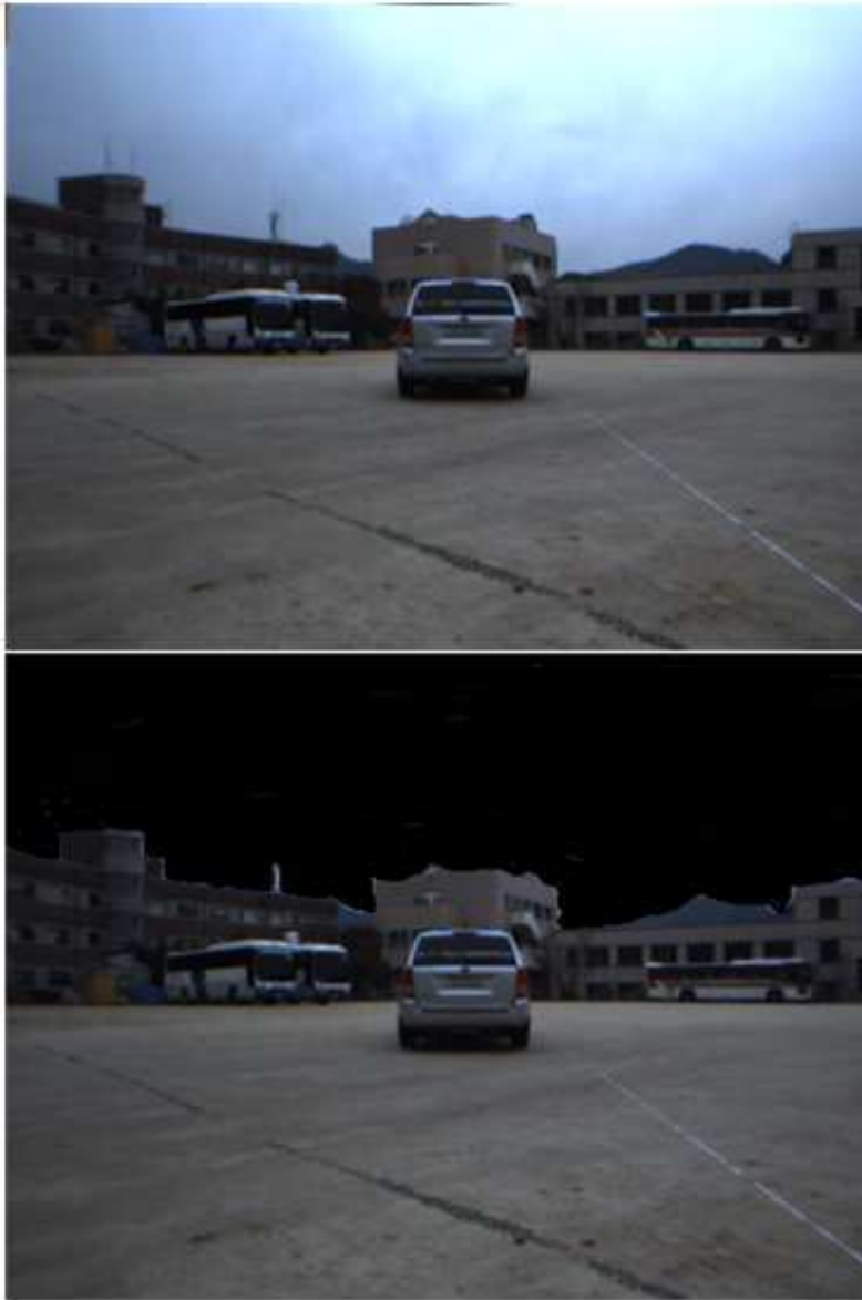
Figure 2.3: Comparison of an original and the same image with the sky removed (shown in black). Based on the image with the sky removed, the region of interest is reduce when generating the disparity map.
