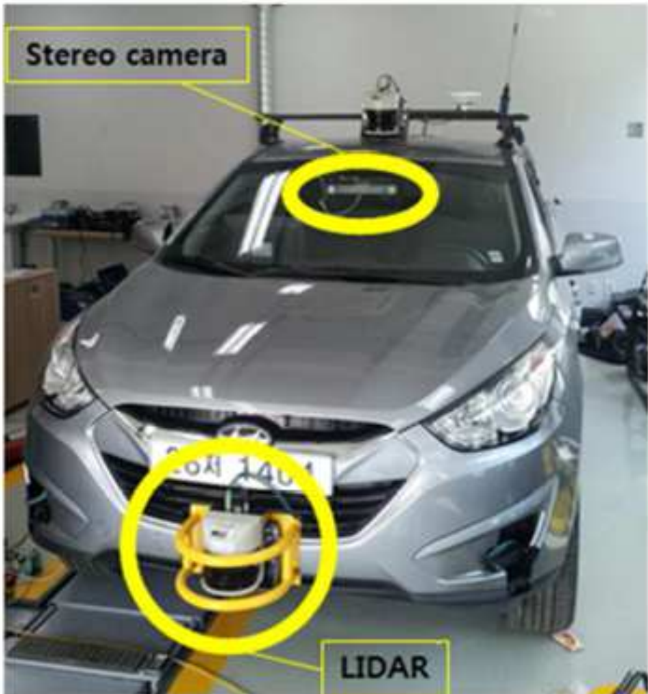
Figure 2.7: SNU autonomous vehicle. The vehicle is equipped with a stereo sensor (indoor), LIDAR (outdoor).
