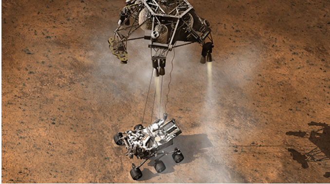
Figure 1.1: Conceptual picture of the descent of NASA’s Curiosity rover to the Martian surface by sky crane for Mars mission launching in 2020 [29].
