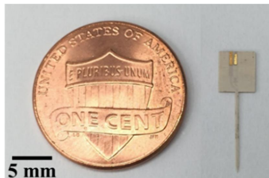
Figure 3.3 Fabricated LCP-based tetrode.
