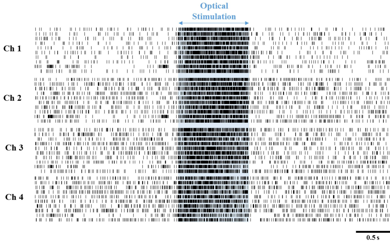
Figure 3.25 Experimental results of in vivo optical stimulation and electrical recording using the LCP-based tetrode: the raster plot.
