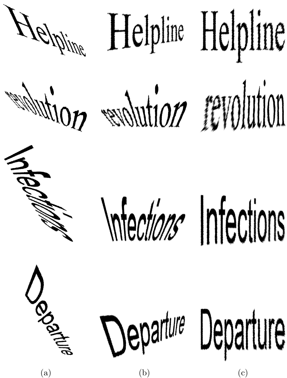
Figure 4.10: Rectification results on English synthetic text images. (a) input distorted image, (b) the conventional method [4], (c) the proposed method.
