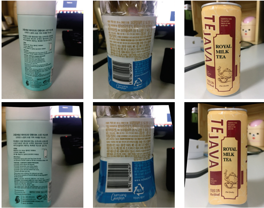
Figure 1.4: Examples of the curved surface dewarping in real scene. the first row: input camera-captured curved surfaces in real scene, the second row: dewarping results of inputs.
