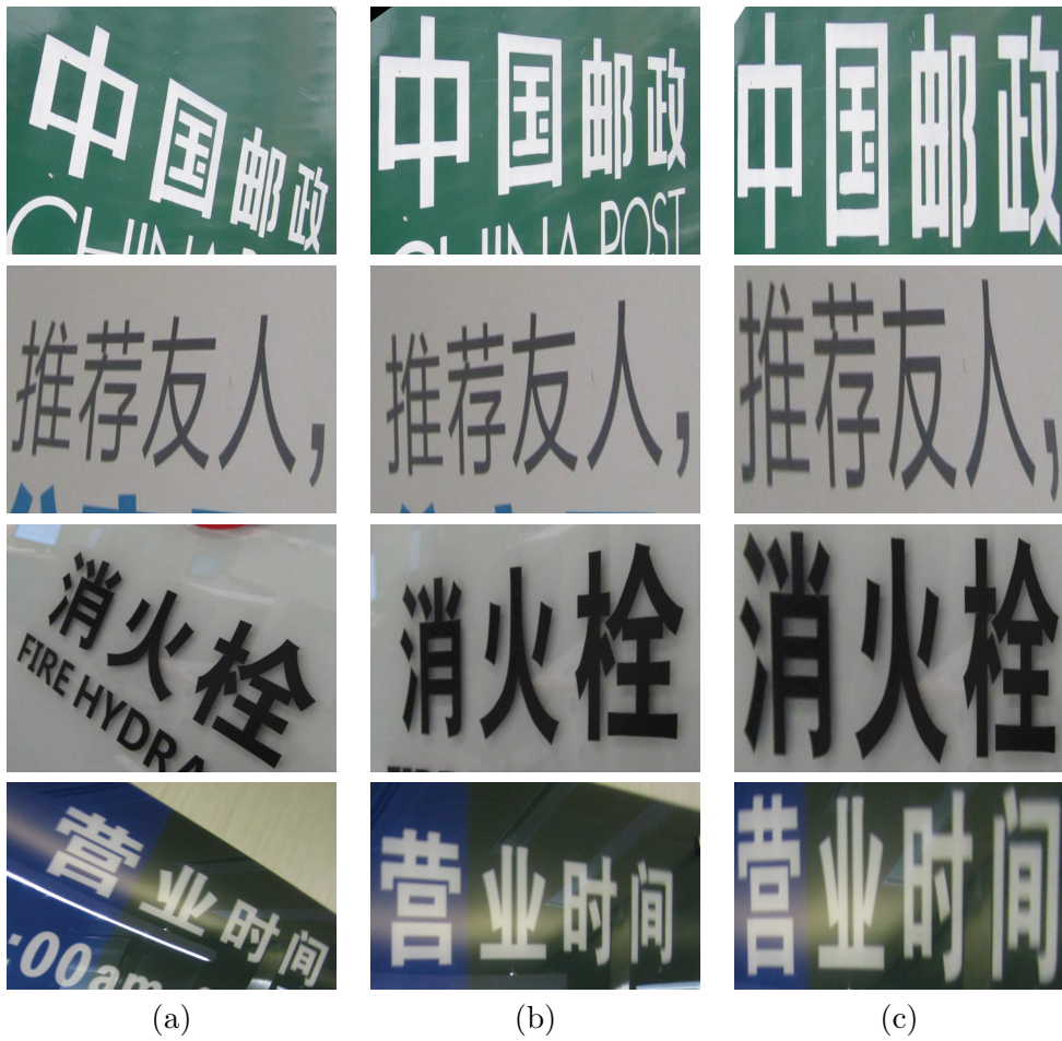
Figure 4.9: Rectification results on Chinese real scene text images. (a) input distorted image, (b) the conventional method [4], (c) the proposed method.
