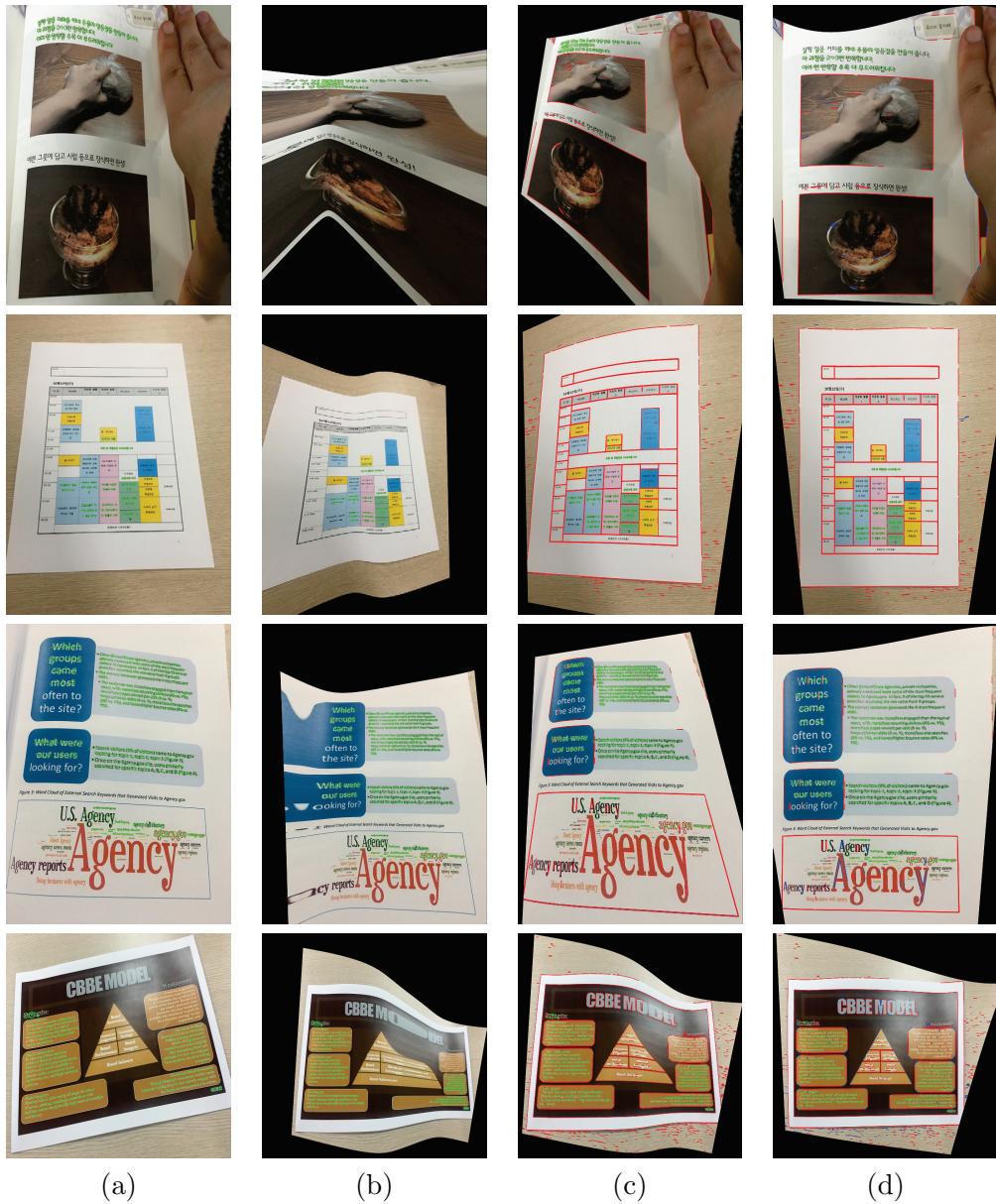
Figure 3.8: Rectified results by minimizing the three cost functions. (a) Input images and (green) text components. (b) Rectified image by minimizing the text-line based term f_{text} , (c) Rectified image by minimizing the text-line based term f_{text} and line segment straightness term f_{str} , and (red) line segments, (d) Rectified image by minimizing the cost function f_{cost} , (red) horizontal/vertical and (blue) non horizontal/vertical line segments.
