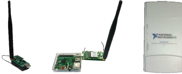
Figure 3.8: TelosB for IEEE 802.15.4 node (left), a set of Raspberry Pi and BCM4356 for BLE node (middle), and NI USB-6210 for power meter (right).
