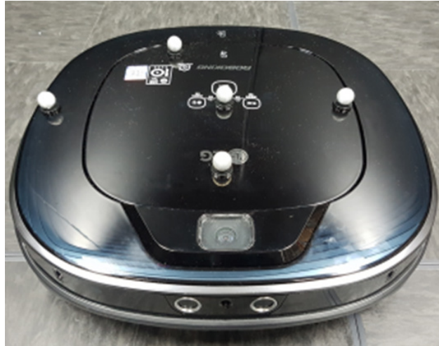
Figure 4.10 Robot platform with markers for motion capture
