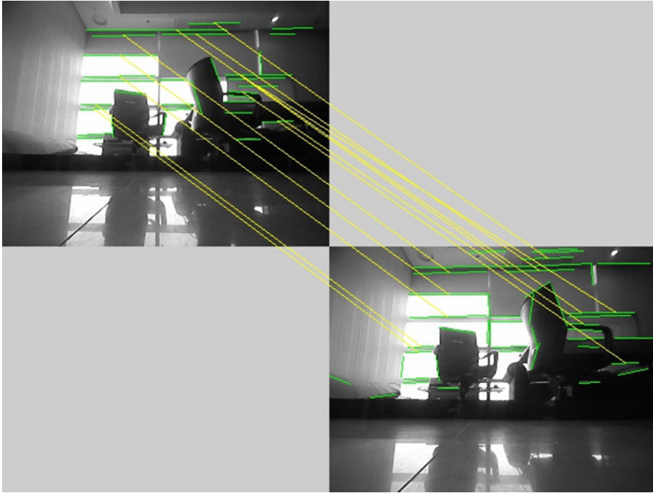
Figure 3.14 Example of line matching result
