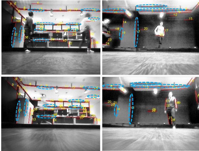
Figure 4.22 Extracted map lines for measuring the mapping error (marked as blue dotted ellipse)
