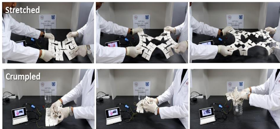
Figure 3.21 Snapshots captured from the video showing the stable operation of the omni-directionally deformable battery at various deformation modes.
