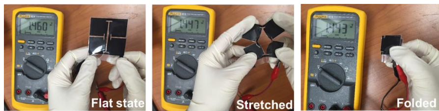
Figure 3.25 Stretching and folding of screen printed level-1 hierarchical auxetic battery.
