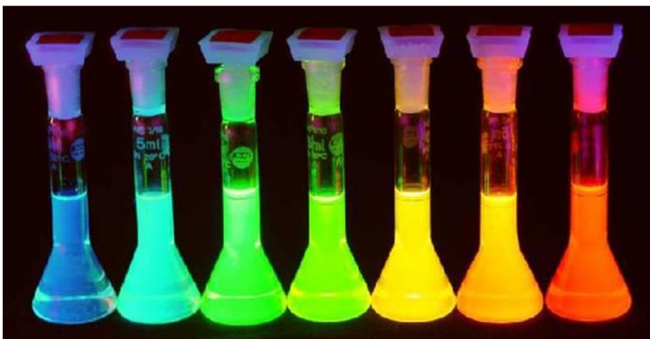
Figure 1.6 This vial contains a solution with monodisperse CdSe quantum dots of different sizes. On the left side, there are small quantum dots ranging from blue to red.
