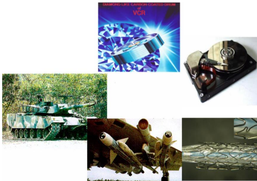
Figure 5.3 Various industrial applications of diamond-like carbon film such as coating for IR window of Tank, Infrared missile, VTR head drum, computer hard disk and stent.
