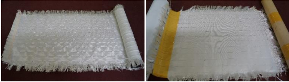
(b) Woven structure (Warp: SMA wire/Glass-fiber, Weft: Glass-fiber)
