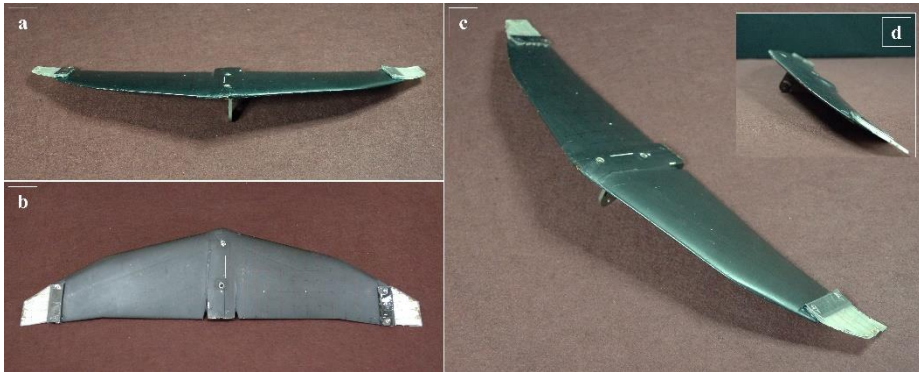
UAV with the mounted morphing winglets; (a) Front, (b) Top, (c) Perspective, and (d) Side view
