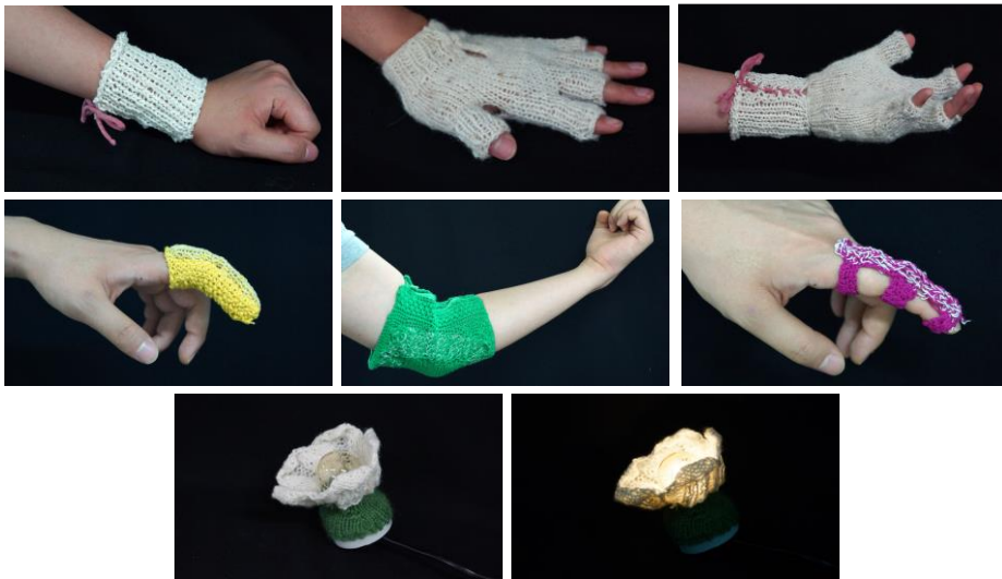
Figure 5-6. Wearable applications using knit actuators
