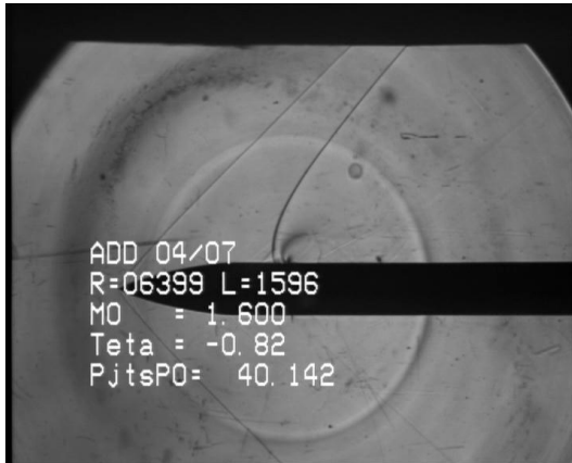
Figure 1.1: Schlieren photograph of side-jet interaction flow field
