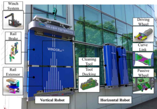
Fig. 1. 4 Building façade maintenance robot, Hanyang University, Korea [11,12]
