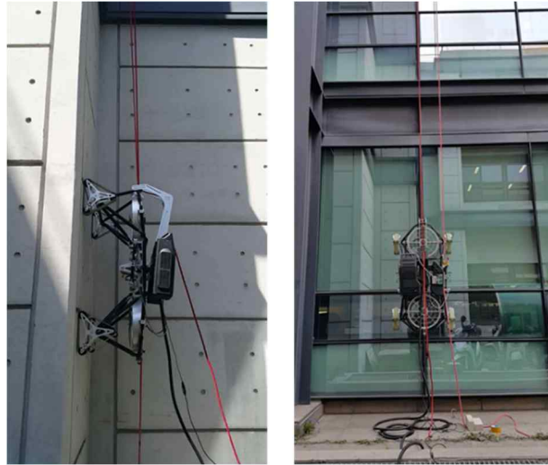
Fig. 5. 1 Experiment of distance data between robot platform and wall of building
