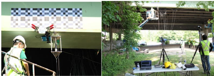
Figure 3. 3 Target and camcorder used for the displacement (FHWA, 2012)
