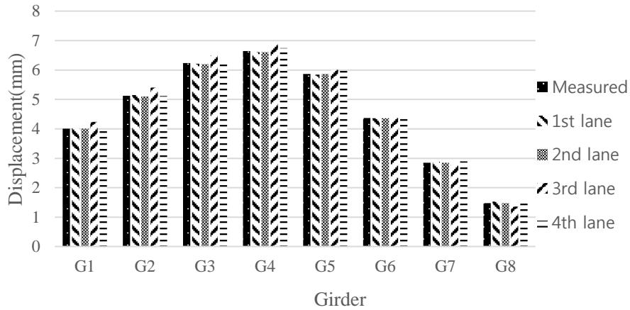
Figure 3. 20 Discrepancies between the static displacement values of the measured and updated model cases
