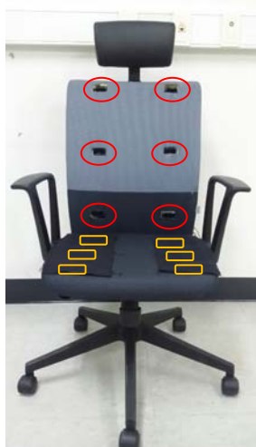
Figure 5. The sensor-based chair. Red circles are the infrared reflective sensors and yellow rectangles are the force sensitive resistors.
