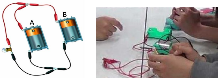
Figure 4.8 Electric circuit with two parallel batteries.
