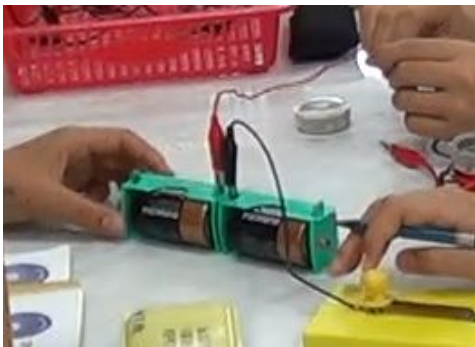
Figure 4.4. Checking whether linking the wires between the two batteries let electricity flow
