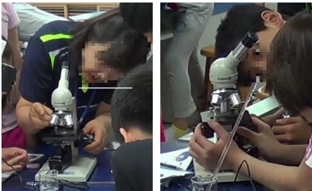
Figure 4.10 Adjusting the focus by moving the stage of the microscope
