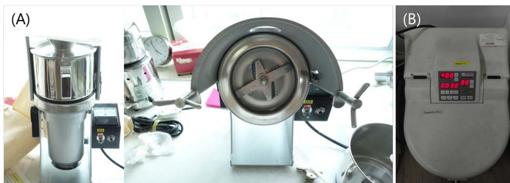
Fig. 1. Two types of grinding machine. (A) Blade grinder (dry grinding, ALG-2) and (B) Ball mill (wet grinding, Planetary Mono Mill PULVERISETTE 6 classic line).
