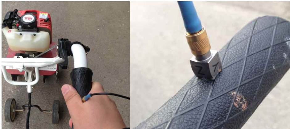
Fig. 22 Accelerometer attached to handle
