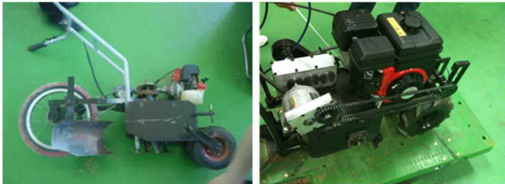
Fig. 6 Horizontal shaft type weeder (left) and crank type weeder (right) developed by Rural Development Administration
