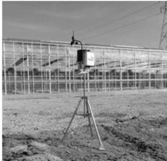
Fig. 8 Installation of sensor for verification experiment; (a) Hobo data logger (Onset computer corp., USA) for measuring the temperature (b) Watchdog 2900ET (Spectrum Technologies Inc., USA) for measuring the outside weather data
