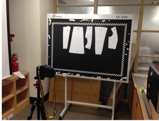
Figure 3.7: The capturing environment that we designed to obtain panel images.
