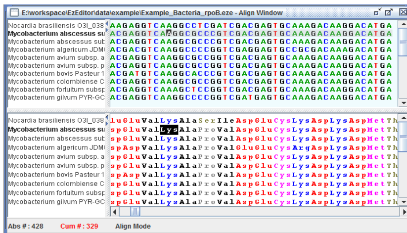
Figure 51. Align Panel of functional coding sequence. Protein sequence alignment is shown in the panel below DNA alignment panel.
