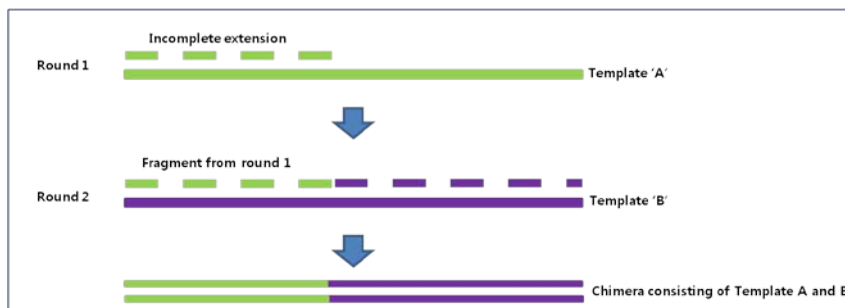
Figure 4. Illustration showing formation of a chimera during PCR reaction.
