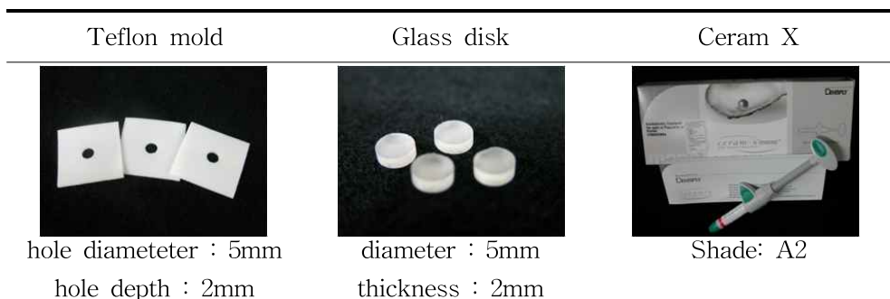
Figure 2. Photographs of teflon mold, glass disk and composite resin used in this study
