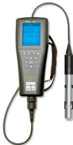
Figure 4.3.1.1: Portable DO meter used for the experiments.
