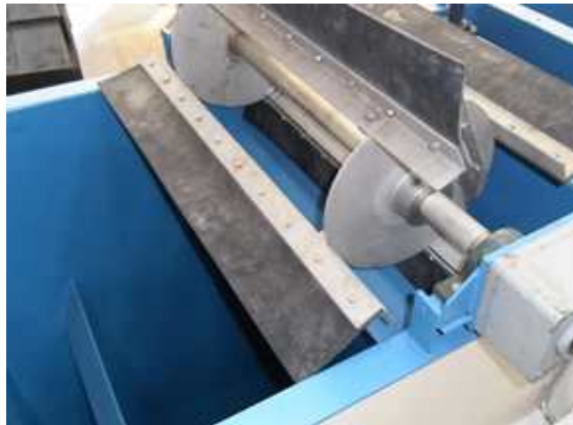
Fig. 2.7 Beach rotating removal system
