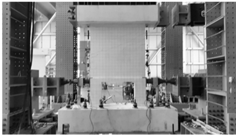
(a) Cyclic loading test setup
