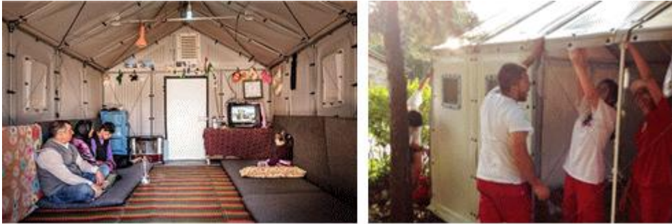
[그림 3-27] Ikea's Flat-pack Refugee Shelter 내부 및 설치과정 (출처: http://www.takepart.com/article/2015/04/10/ikea-refugee-shelters-iraq http://www.bettershelter.org/product )
